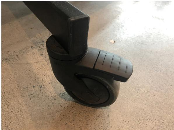
This image shows a castor with the brake disengaged. To engage the brake, push the tip of the plastic lever down with your foot until it clicks. The image below shows how far you must push the lever for it to engage.
