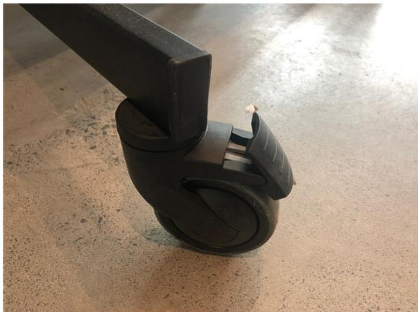
This image shows a castor with the brake engaged. To disengage the brake, push the top of the plastic lever backwards and downwards until it releases and springs back to the disengaged state shown in the image above.
